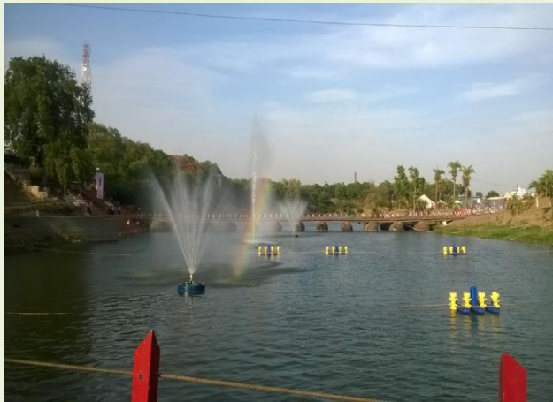
Fountains and paddle wheel aerators at Mangalnath Ghat for River water purification
