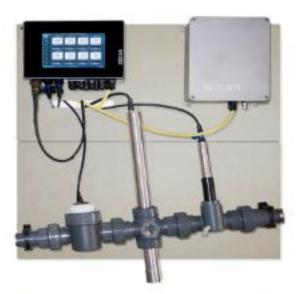
The fully modular micro::station combines s::can instruments to a compact and versatile system. It presents a complete solution, as the user only has to connect water supply and -discharge ("plug & measure") in order to receive at no extra cost a previously unheard variety of immediately available information and parameters.
